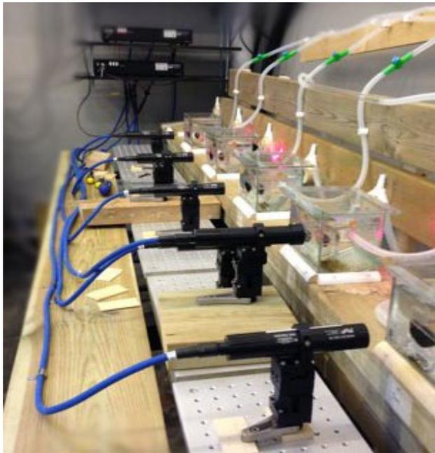
The laser sensor can measure accurately the feeding habit of the mussels by measuring the particle size, particle count and the flow speed both for the intake and outflow of each mussel. By subtracting the mass out from the mass in, the amount of the material taken by the mussel can be calculated. See the figure and graph:
