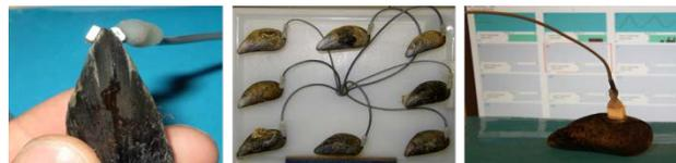
The modernization of these sensors led to the development of 2nd generation biosensors. Limitations with these sensors, such as low sensitivity to low-dose exposure and complex mixtures of toxic substances, generated a need for a next generation of biosensors that are more sensitive and can be integrated into the IO-center (Integrated Operations) of companies. In addition, the new technology measures fitness end-parameters that can be utilized in established environmental risk assessment models.
